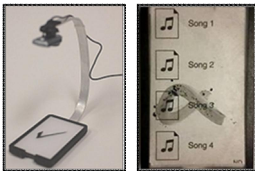
Figure 2: Gesture rig for collecting and recording gestures (left) and an example gesture for the action “delete” (right).
